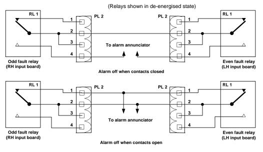
(Switch SW6 set for fault signal operation)
